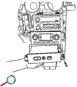
3. Install the communication interface module screws.
